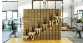
3D-printed earth wall with integrated timber stairs (2). © IAAC
