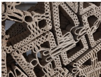
3D-printed cellulose panels interlocked as screen. © CITA
