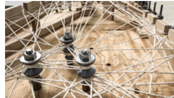
Testing mechanical properties of the flax material system_detail. © ITKE/ICD
