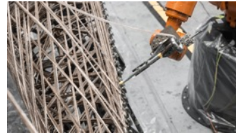
Robotic winding of flax fibre prototype. © ITKE/ICD
